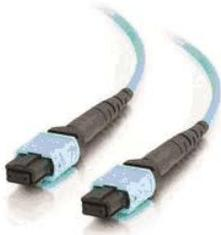
Cables Unlimited offers Corning fiber assemblies using Multi-fiber Termination Push-on (referred to as MTP) connectors designed by USConec. This compact design allows high-density connections between network equipment. A simple push-pull latching mechanism provides easy insertion and removal. Where space is an issue, the MTP allows for more connectors on the overcrowded faceplate, thus reducing the footprint of the systems. It will interface with current MPO connectors. It will
