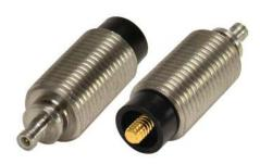
Sometimes the most effective and economical design for a piece of equipment requires a custom adapter to function. Aviel Electronics recently designed such an SMB jack adapter. The CO-SMB-JKMA-3P01 is a panel-mount with a modified interface to allow external sealing and a .060 axial shift when mated with a standard off-the-shelf SMB plug. This special adapter allows RF electrical connection to a non-standard unit,
