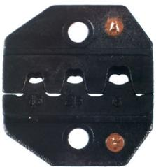
For non-insulated open barrel terminal from 0.5 to 6 sq.mm. AWG 22-18, 16-14, 12-10
