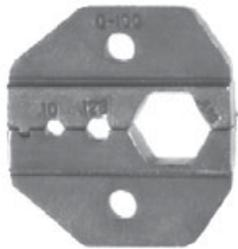
For RG-8/U, RG-213/U, RG-214/U, and Belden 9913 cables, cavity dimensions: .100", .128" and .429". The .128" cavity crimps the center pin on Belden 9913 cable.
