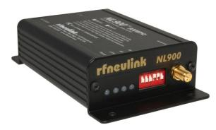
San Diego, CA – The NL900PRO transceiver is a Frequency-Hopping Spread Spectrum (FHSS) radio designed for license-free operation in the 900 MHz ISM band. The radio sustains a standard asynchronous serial data stream between two or more radios out of the box. Housed in a compact and rugged die-cast enclosure, the radio is equipped to replace miles of serial cable using a selectable RS232, RS485, or RS422 interface.
