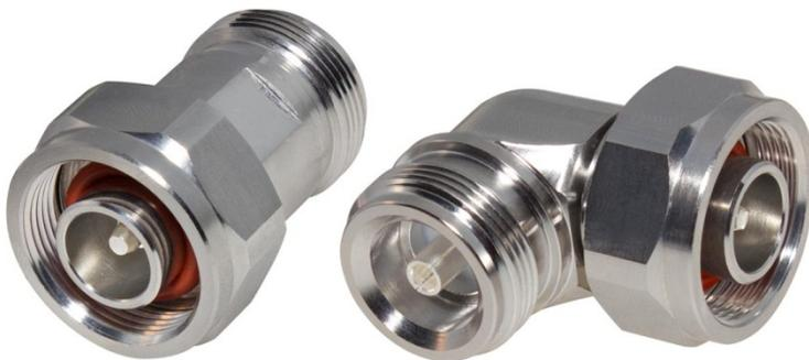
In addition to 8 variations of 4.1/9.5 (Mini) DIN to N type and 7/16 DIN adapters, RF Industries developed a 4.1/9.5 (Mini) DIN male to female right angle and straight adapters. The 4.1/9.5 (Mini) DIN is essentially a compact version of the 7-16 DIN with similar electrical performance. Applications include wireless infrastructure sites, indoor/outdoor DAS (Distributed
