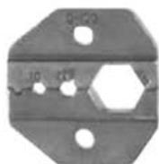
For RG-8/U, RG-213/U, RG-214/U, and Belden 9913 cables, cavity dimensions: .100", .128" and .429". The .128" cavity crimps the center pin on Belden 9912 cable.
