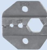
The **RFA-4005-02** die set is used to crimp RG-8/U, RG-213/U, RG-214/U, and Belden 9913 cables. Cavity dimensions: .100", .128", & .429".
