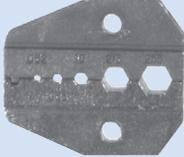
The **RFA-4005-01** die set is used to crimp RG-58/U, RG-59/U, RG-142/U, RG-8X, Proflex and various video cables. Cavity dimensions: .052", .068", .100", .213", & .255".
