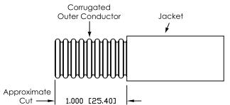
**Step 2. Make second jacketing cut.** Scribe line on ridge of exposed corrugated outer conductor. Line must be at least 13/32 in (10mm) from end of cable. Remove jacket to dimension shown using straight-edged piece of heavy paper wrapped around cable to guide cut.
