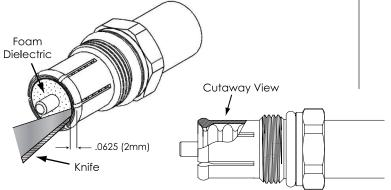
**Step 7. Inspect contact surface.** Thread outer body to clamping nut and tighten with wrenches. Turn outer body only; do not turn clamping nut. Disassemble connection to inspect for good metal-to-metal contact of flared outer conductor.
