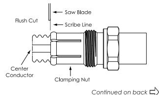
RF Connectors, A Division of RF Industries 7610 Miramar Road, San Diego, CA 92126; (800) 233-1728; (858) 549-6340; fax: (858) 549-6345 www.rfindustries.com; rfi@rfindustries.com **Step 5. Trim center conductor.** Cut center conductor to length shown. Use file to deburr cut end of center conductor.
