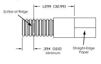
**Step 3. Install gasket.** Add thin O-ring gasket to second fully-exposed corrugation groove from jacket. Apply thin coating of silicone grease to outer surface of gasket and gasket lead chamfer in clamping nut using finger tip. Do not allow silicone grease on threads of clamping nut.
